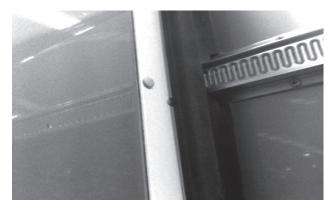
2. Remove the screw located at the top of the unit slide mechanism.
